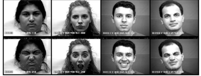
Fig. 2. Extracted feature points.
