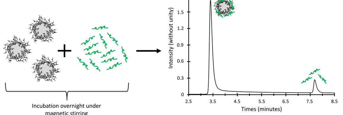
Figure 1. Chromatogram showing the retention times of LNCs (3.5 minutes) and NFL (7.7 minutes) on size exclusion column.
