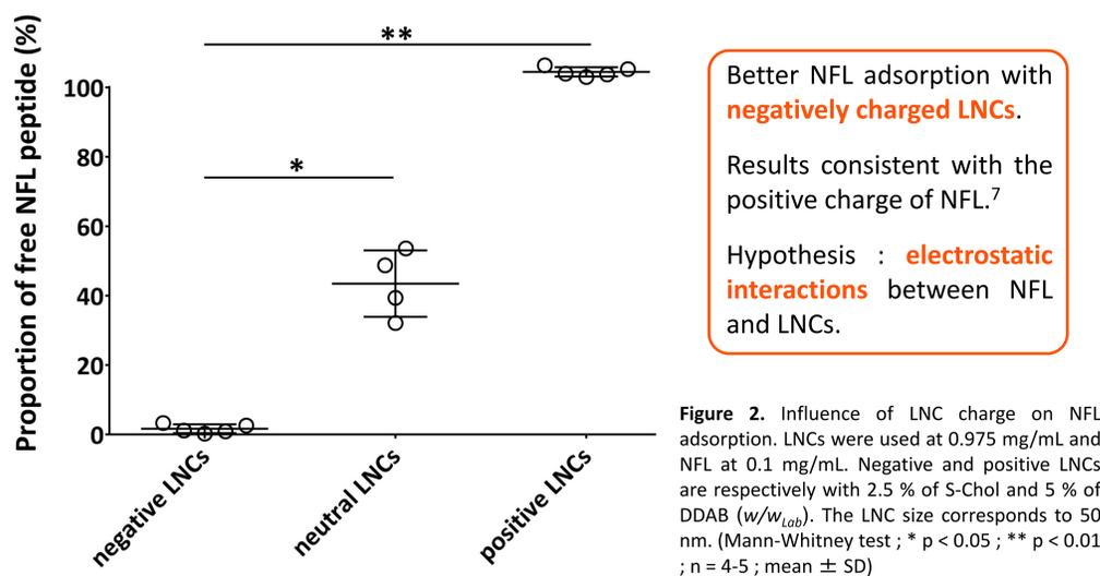
Figure 2. Influence of LNC charge on NFL adsorption. LNCs were used at 0.975 mg/mL and NFL at 0.1 mg/mL. Negative and positive LNCs are respectively with 2.5 % of S-Chol and 5 % of DDAB ( $w/w_{Lab}$ ). The LNC size corresponds to 50 nm. (Mann-Whitney test ; \*  $p < 0.05$  ; \*\*  $p < 0.01$  ;  $n = 4-5$  ; mean  $\pm$  SD)
