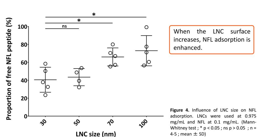
Figure 4. Influence of LNC size on NFL adsorption. LNCs were used at 0.975 mg/mL and NFL at 0.1 mg/mL. (Mann-Whitney test ; \*  $p < 0.05$  ; ns  $p > 0.05$  ;  $n = 4-5$  ; mean  $\pm$  SD)
