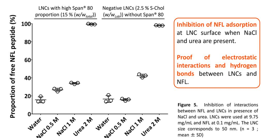
Figure 5. Inhibition of interactions between NFL and LNCs in presence of NaCl and urea. LNCs were used at 9.75 mg/mL and NFL at 0.1 mg/mL. The LNC size corresponds to 50 nm. ( $n = 3$  ; mean  $\pm$  SD)
