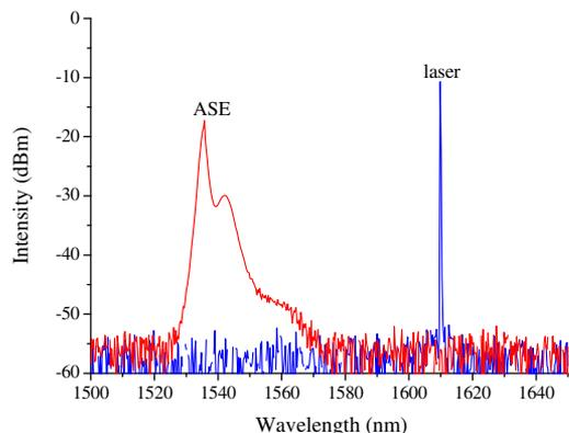
Fig. 2. Optical spectra of the laser and ASE.
