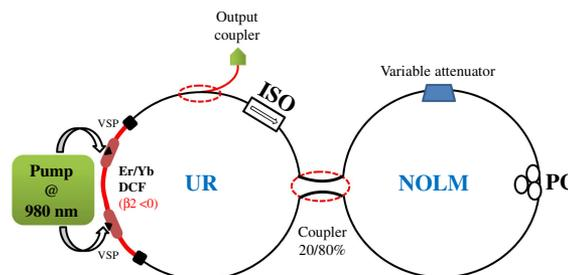
Fig. 1. F8L schematic.
