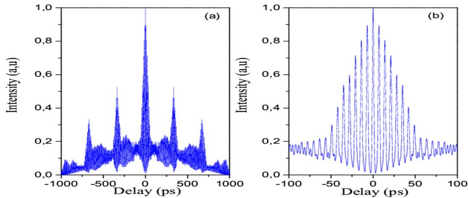
Fig. 6. Autocorrelation trace of a diphasic mixture of solitons(a), Zoom (b), (reconstructed).
