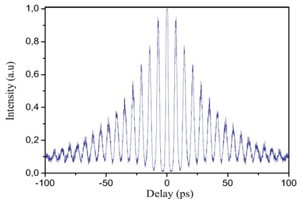
Fig. 3. Autocorrelation trace (experiment).
