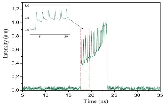
Fig. 2. Temporal trace of the soliton distribution (experiment).
