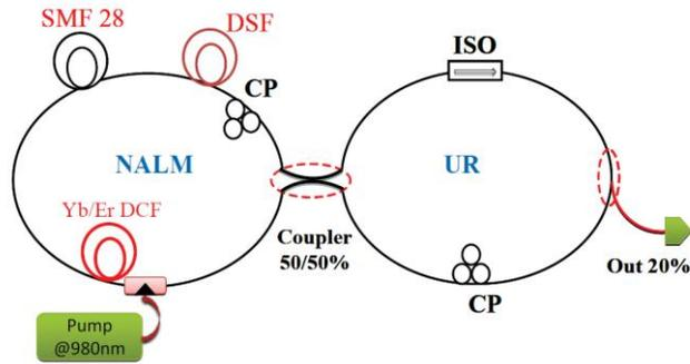
Fig. 1. Experimental setup. DCF: double-clad fiber; DSF: dispersion-shifted fiber; ISO: optical isolator; PC: polarization controller. NALM: nonlinear amplifying loop mirror, UR: unidirectional ring.
