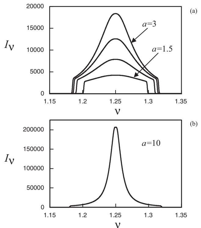
FIG. 5. Dependence of the spectral profile of a steady-state pulse on the pump power  $a$ . (a) The pump power changed with a step  $\delta a = 0.5$ . (b)  $a = 10$ . All other parameters are the same as in Fig. 4.
