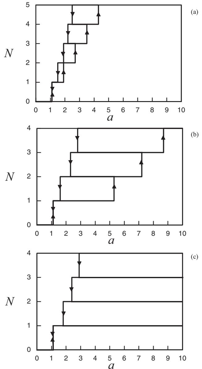
FIG. 2. Number of pulses  $N$  vs pump power  $a$ . (a)  $D_i = -20$ . (b)  $D_i = -25$ . (c)  $D_i = -28$ . For all figures,  $D_r = 1$ ,  $p = 1$ ,  $q = 18$ ,  $\sigma_0 = 1$ ,  $p_2 = 3$ ,  $q_2 = 0$ , and  $b = 0.01$ .
