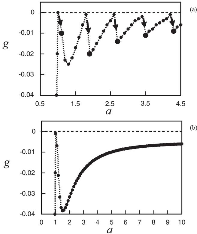
FIG. 3. Dependence of the total amplification  $g$  on the pump power  $a$ . (a) Usual passive mode locking. The arrows point to jumplike transitions from steady states with  $g = 0$  to the state with  $g < 0$  designated by large black circles.  $D_i = -20$ . (b) Passive mode locking under dissipative soliton resonance conditions. The dependence  $g = g(a)$  corresponds to the lowest branch in Fig. 2(c).  $D_i = -28$ . Other parameters are the same as in Fig. 2.
