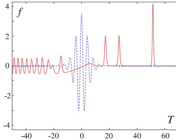
Fig. 2 – (Color online) Wave profile showing the formation of three unipolar half-cycle solitons from a FCP input. Dashed line is the FCP input ( $Z = 0$ ), solid line is output ( $Z = 3$ ). The dimensionless parameters are: amplitude  $\mathcal{A} = 3.5$ , angular frequency  $\omega = 1.5$ , carrier-envelope phase  $\psi = 0$ , and duration  $T_0 = 5.33$  (after [49]).
