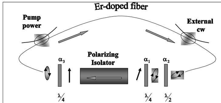
Figure 4. Schematic representation of a passive mode-locked erbium-doped fiber laser with a nonlinear polarization rotation technique and an external cw injection.
