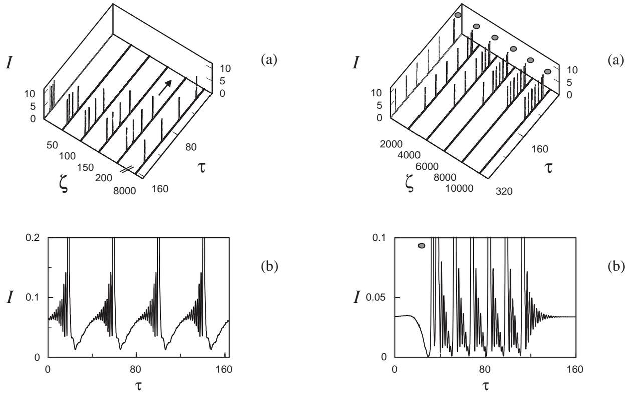
Figure 7. Dependence of the intensity distribution  $I(\tau)$  on the number of round trips  $\zeta$  in a passive mode-locked laser with an injected cw. Regime of a soliton repulsion. (a) Transient process. (b) Steady state (the scale is enlarged).  $K = 40$ ,  $P = 0.1$ ,  $l \approx 164$ .
