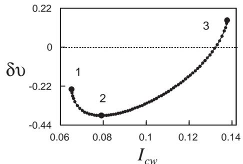
Figure 6. Soliton velocity  $\delta v$  vs the intensity  $I_{cw}$  of the injected cw.  $K = 40$ .
