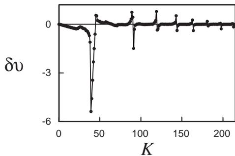
Figure 5. Soliton velocity  $\delta v$  vs the frequency parameter  $K$  of the injected cw.
