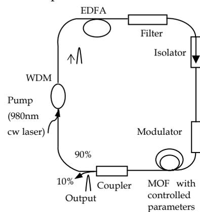
Figure1: Set up of the fiber ring laser
