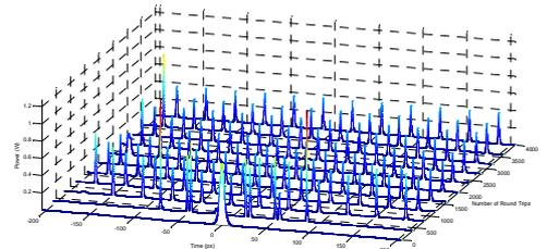
Figure 7: Numerically calculated pulse evolution in actively ring fiber laser:  $g_0=2\text{m}^{-1}$  and  $E_s=5\text{pJ}$ .
