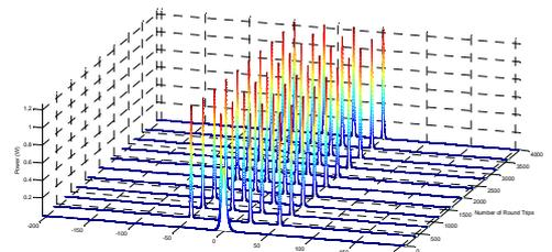
Figure 8: Numerically calculated pulse evolution in actively ring fiber laser,  $\gamma_{\text{MOF}}=0.0012/\text{w/m}$
