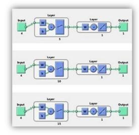
Figure 2: Feed-Forward Back Propagation Networks Used: Once with 4 Inputs and Second With 2 Inputs, and Each with 5, 10 & 15 Neurons in the Hidden Layer
