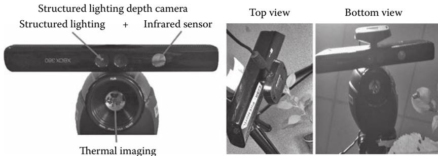
**Figure 9.9** (See color insert.) Left: The anatomofunctional imaging system in this chapter is composed of a depth camera using the 2D structured lighting (binary dot pseudorandom grid) method and a thermal imaging. Right: An acquisition on a plant is done by one shot taken in plant top view.
