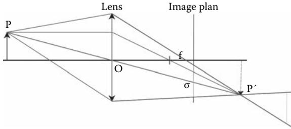
Figure 9.3 Principle scheme of blur in camera.
