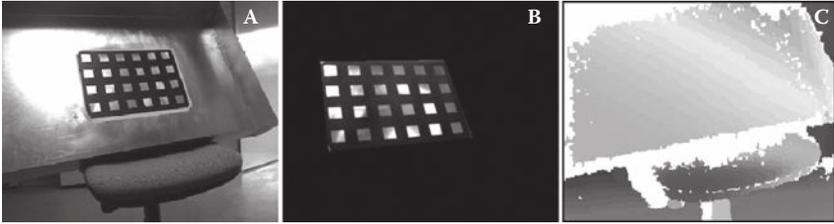
**Figure 9.10** (See color insert.) A calibration scene. (a) The RGB image of the calibration chessboard on the metallic plane. (b) The thermal image of the calibration chessboard on the metallic plan. (c) The disparity map of the calibration chessboard plan.
