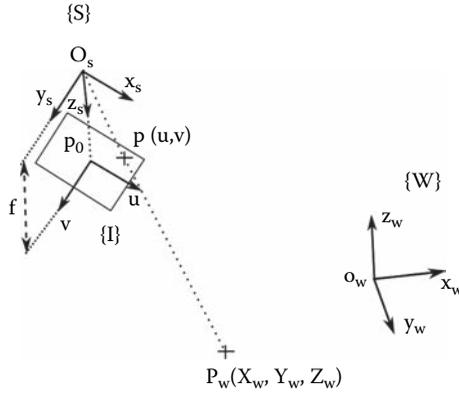
Figure 9.7 The principle scheme of the pinhole model.
