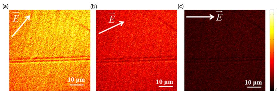
FIG. 3. SHG images as a function of polarization. 3(a) Polarization at  $50^\circ$  with respect to p polarization, corresponding to SHG maximum. 3(b) polarization at  $25^\circ$  with respect to p polarization, corresponding to intermediate SHG signal. 3(c) p polarization corresponding to SHG minimum.
