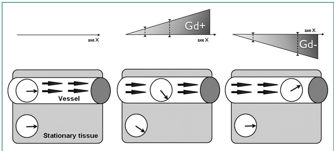
**Figure 1.** Diagrammatic representation of the principle of phase-contrast velocimetry MRI. When the first phase of the bipolar gradient ( $Gd+$ ) is applied, spins shift phase depending on their position on the x-axis. When the second, same intensity and duration but reverse polarity, gradient ( $Gd-$ ) is applied, the phase shift of stationary protons is cancelled out whereas the phase shift of moving protons becomes proportional to their speed.
