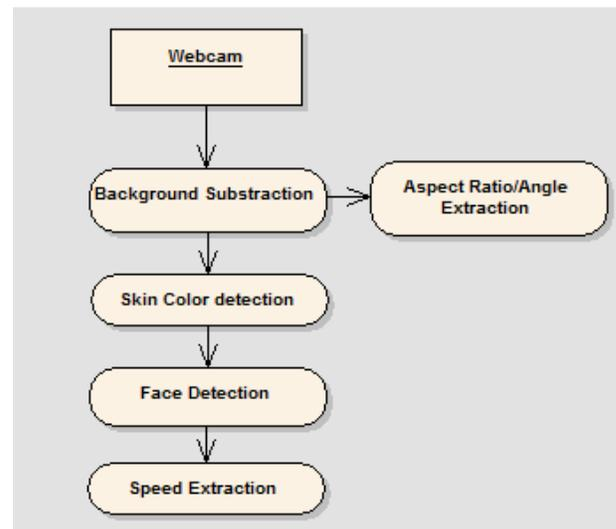
**Figure 2.** Overview of the webcam monitoring system
