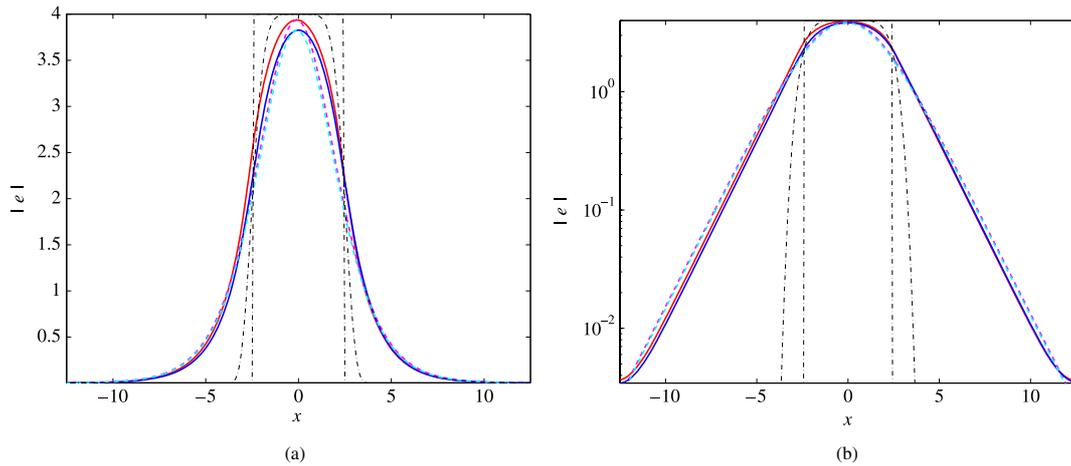
**Figure 2.** Transverse electric field amplitude profile in both linear (a) and logarithmic (b) scales. Solid curves: numerical resolution of the Maxwell–Bloch equations for super-Gaussian (upper, red curve) and top-hat (lower, blue curve). The dashed curves are  $\text{sech}^2$  fits. The dash-dot curves are proportional to the top-hat and super-Gaussian pumpings.
